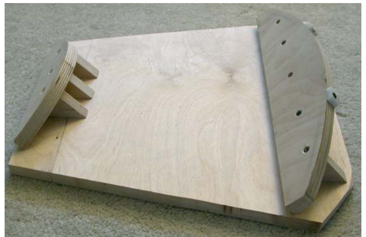
I'm fortunate to live at 45.78 degrees north latitude so both bearings are mounted on 45 degree angles.
