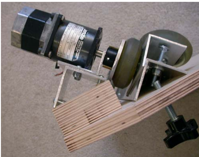
Here is the motor mounting detail. The motor is supported by the drive wheel, and also by the mounting bracket.
