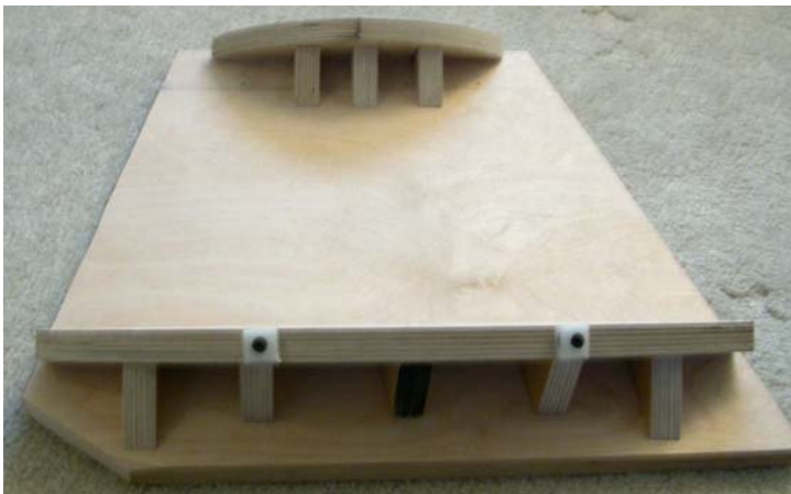
Here is a view of the bottom side of the upper platform. The north bearing is at the front of the photo and the south bearing is at the back of the photo.
