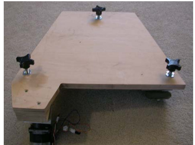
This photo shows the bottom of the lower platform. I used 3/8" knobs to level the platform. The adjusting knobs are below the centerlines of the north and south angle/wheel assemblies. In the next photo you can see the adjustment knob below the angle.
