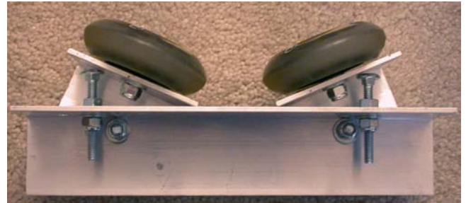
This is the back side of the south angle/wheel assembly. Notice that I used carriage bolts to support the back side of the angles that mount the wheels.
